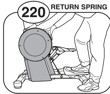
To attach side panel, push foot pad to floor and locate side panel.
