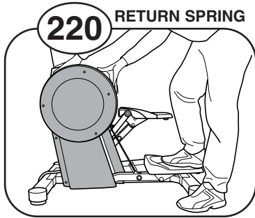
To remove side panel, push foot pad to floor (if necessary) and detach side panel.
